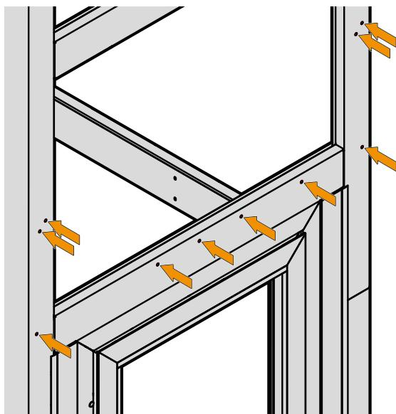
7. Accurately apply silicone **G** in the area in contact with the structure.
