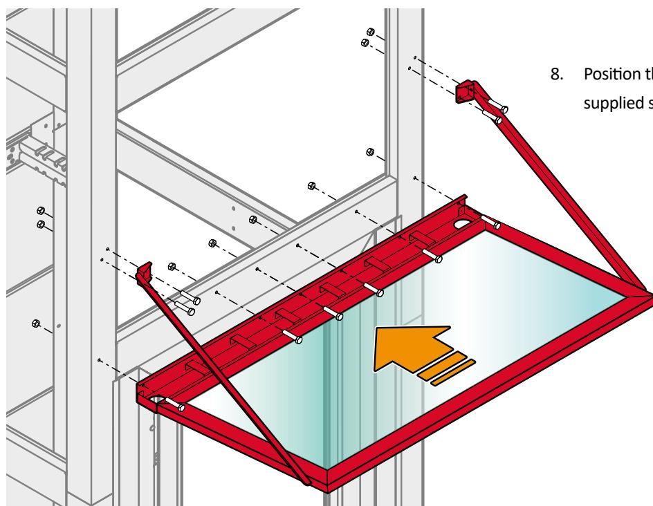
8. Position the canopy **H** and secure it with the supplied screws.
