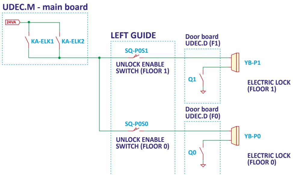
For increased safety the main board checks if the enabling contacts (SQ-PoS, SQ-P1s) are glued or stuck. These are the steps of the test:
